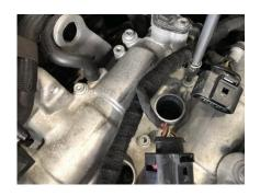
Remove the 2 bolts on the valve cover using an allen 5 bit.
