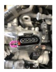
Using a small flat head screw driver slide the pink tab out of the coil pack connector.
