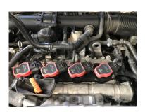
Place the 4 R8 coils in the adapter, connect the 4 connectors on each coil and push them down to fit snug.
