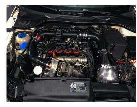
Push the breather hose on to the intake nipple and then using pliers position the hose clamp properly.
