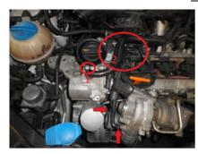
Remove the bolt holding the plastic vent(1) fitting using a T30 bit and pull up the vent tubing out of the valve cover. Then and rotate it out of the way(2).
