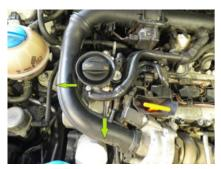
Remove the small breather hose clamp from the intake tube using pliers to release the clamp.
