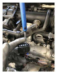
Using an appropriate VW Connector pin removal tool pry the only small diameter wire (Position No4 in stock form) out of the connector (pull from the back side).
