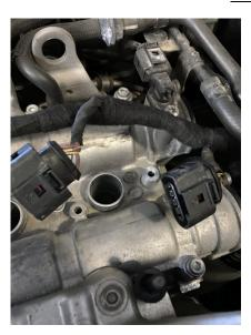
Place the provided spacers on the two blank bolt holes and position the RTMG R8 coil adapter on the valve cover.
