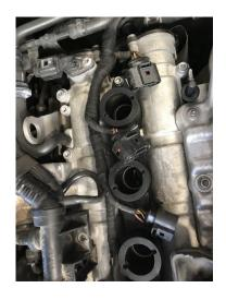
Place the RTMG Performance coil adapter over the spacers and insert the two M6 bolts provided in the package but don't tighten them fully.
