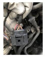
Once you have clicked all the wires in to place properly slide the pink retainer clip in the reverse order of removal. It should go in without resistance and click. The coil pack connector wires should be like the photo.
